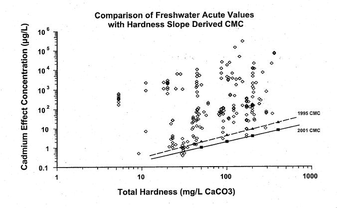
Figure 1. Comparison of All Table 1 Freshwater Acute Toxicity Test EC50s and LC50s with the Hardness Slope Derived CMC. (2001 CMC: solid line; 1995 CMC: dashed line)
