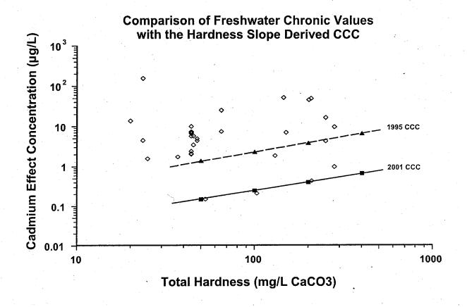
Figure 4. Comparison of All Table 2 Freshwater Chronic Values with the Hardness Slope Derived CCC. (2001 CCC: solid line; 1995 CCC: dashed line)
