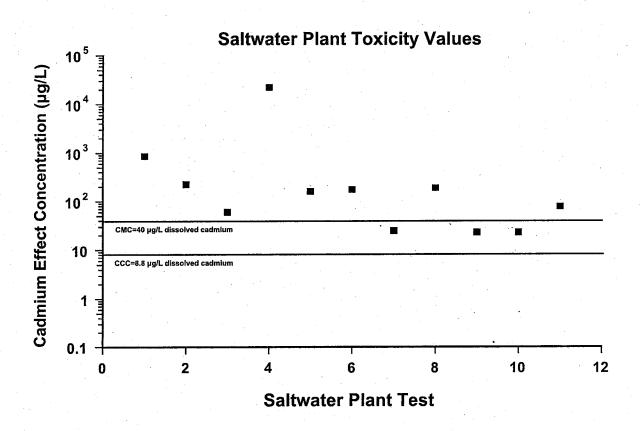
Figure 7. Comparison of Saltwater Plant Toxicity Values (Table 4) and Saltwater CMC and CCC Values.
